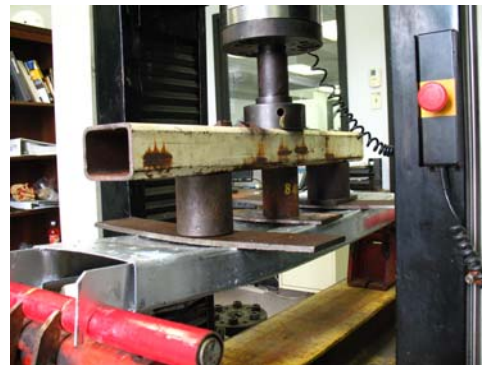
UDL failure at 6,715 lbs.
