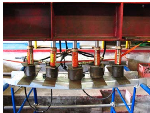
UDL failure at 6,315 lbs.
