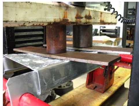
UDL failure at 7,970 lbs.
