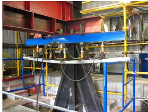
UDL failure at 2,330 lbs.
