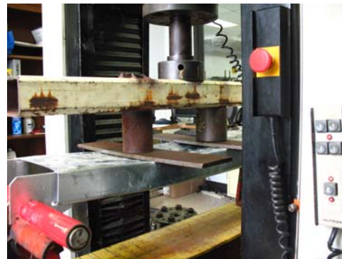
UDL failure at 7,060 lbs.
