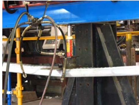
Point load failure at 1,475 lbs.
