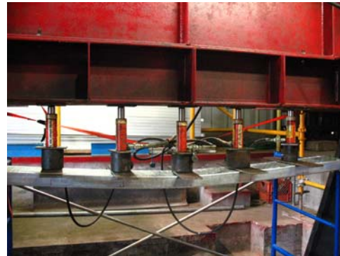
UDL failure at 3,030 lbs.
