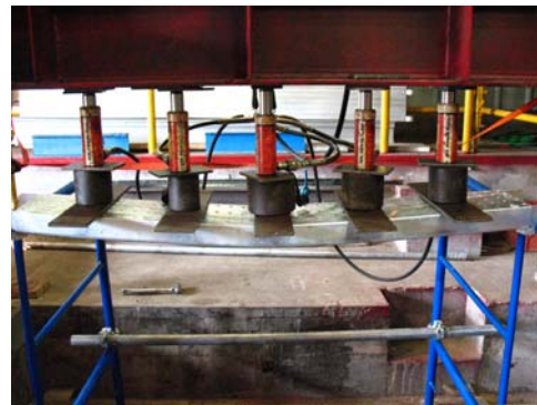
UDL failure at 4,545 lbs.
