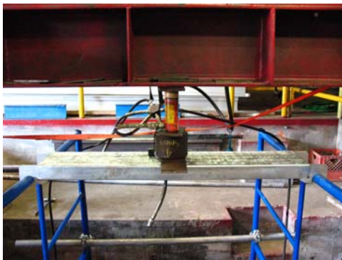
Point load setup
