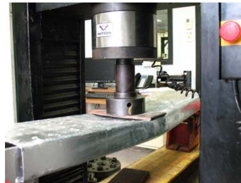
Point load failure at 3,900 lbs.
