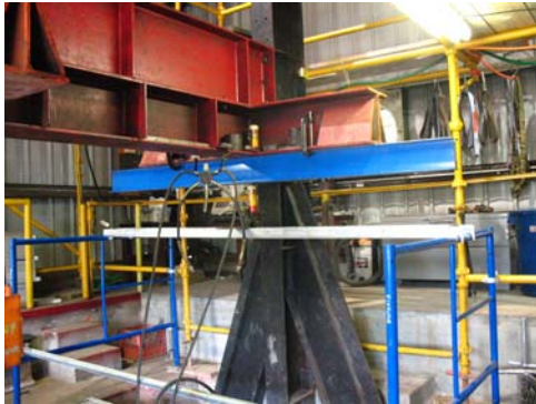
Point load setup
