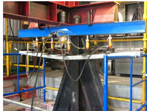
UDL failure at 2,330 lbs.
