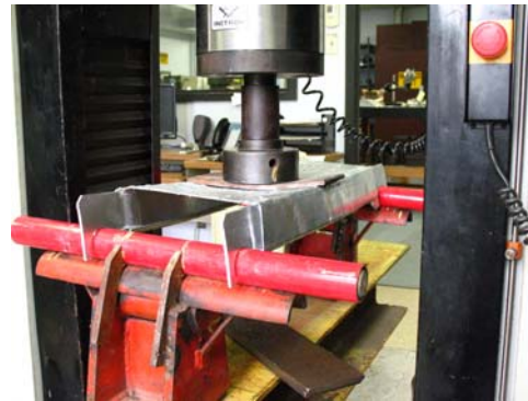
Point load failure at 5,715 lbs.
