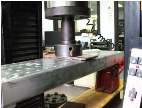
Point load setup
