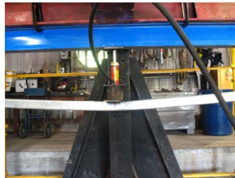
Point load failure at 1,100 lbs
