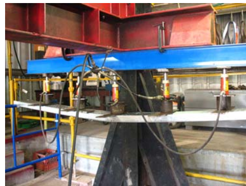
UDL failure at 1,535 lbs
