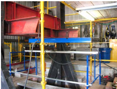
Point load setup
