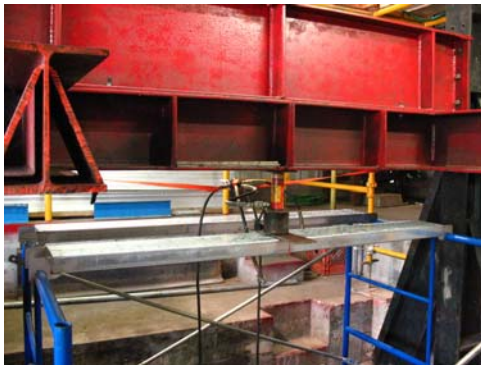
Point load setup
