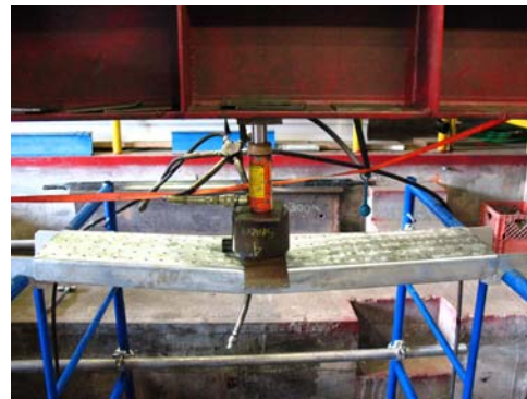
Point load failure at 3,415 lbs.
