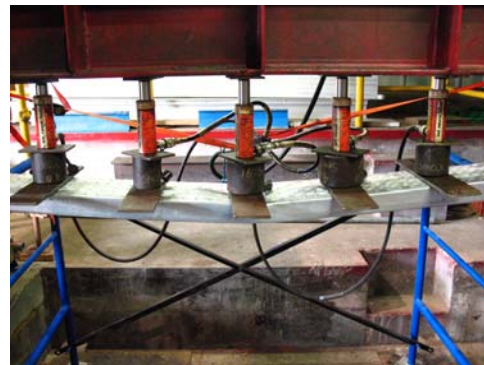
UDL failure at 3,685 lbs.
