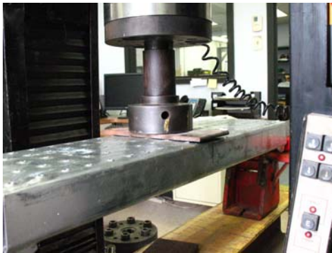
Point load setup
