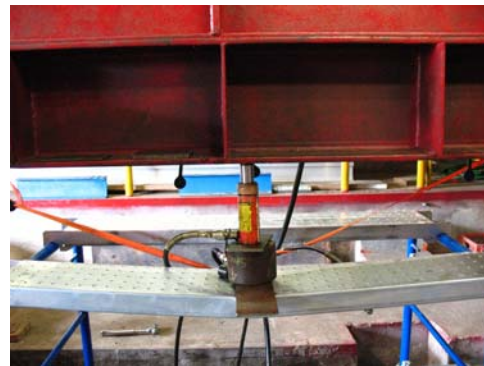
Point load failure at 2,790 lbs.
